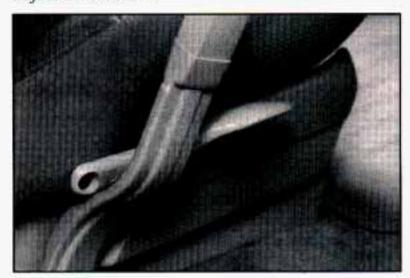
You can adjust the seatback by lifting the lever. Release the lever to lock the seat back where you want it. Pull up on the lever and the seat will go to an upright position.
